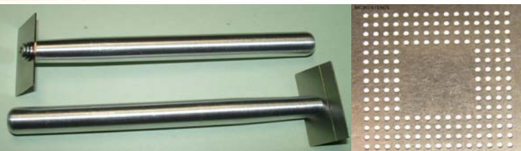
Stapula for BGA paste/flux application. 19cm length
